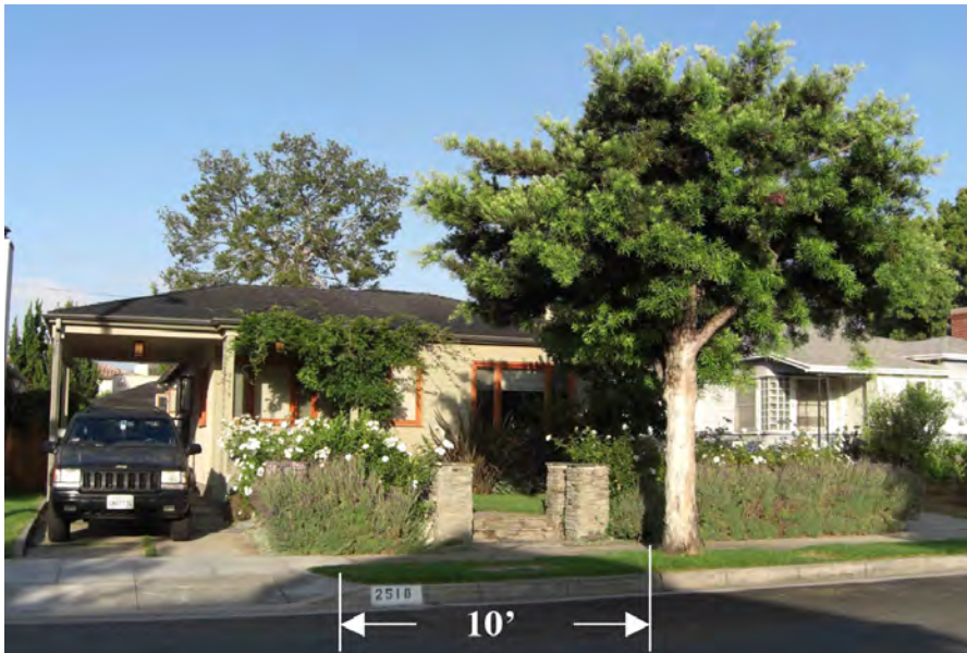
Fig A8 - New driveways must be ten feet (10') minimum from the existing street tree.
