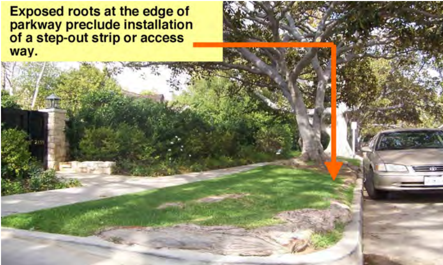
Fig A12 - Exposed surface roots growing against the perimeter of a parkway do not allow for the addition of a step-out strip.
